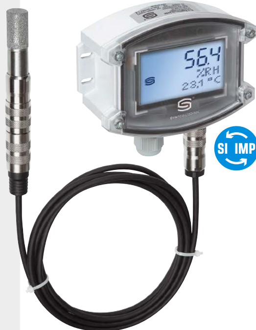
RPFF-25 / RPFTF-25 ( \pm 1.8\% ) pluggable measuring head with metal sinter filter and display
